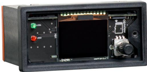
Figure 7: EOR-1DS with demounted front plate for SD card access
